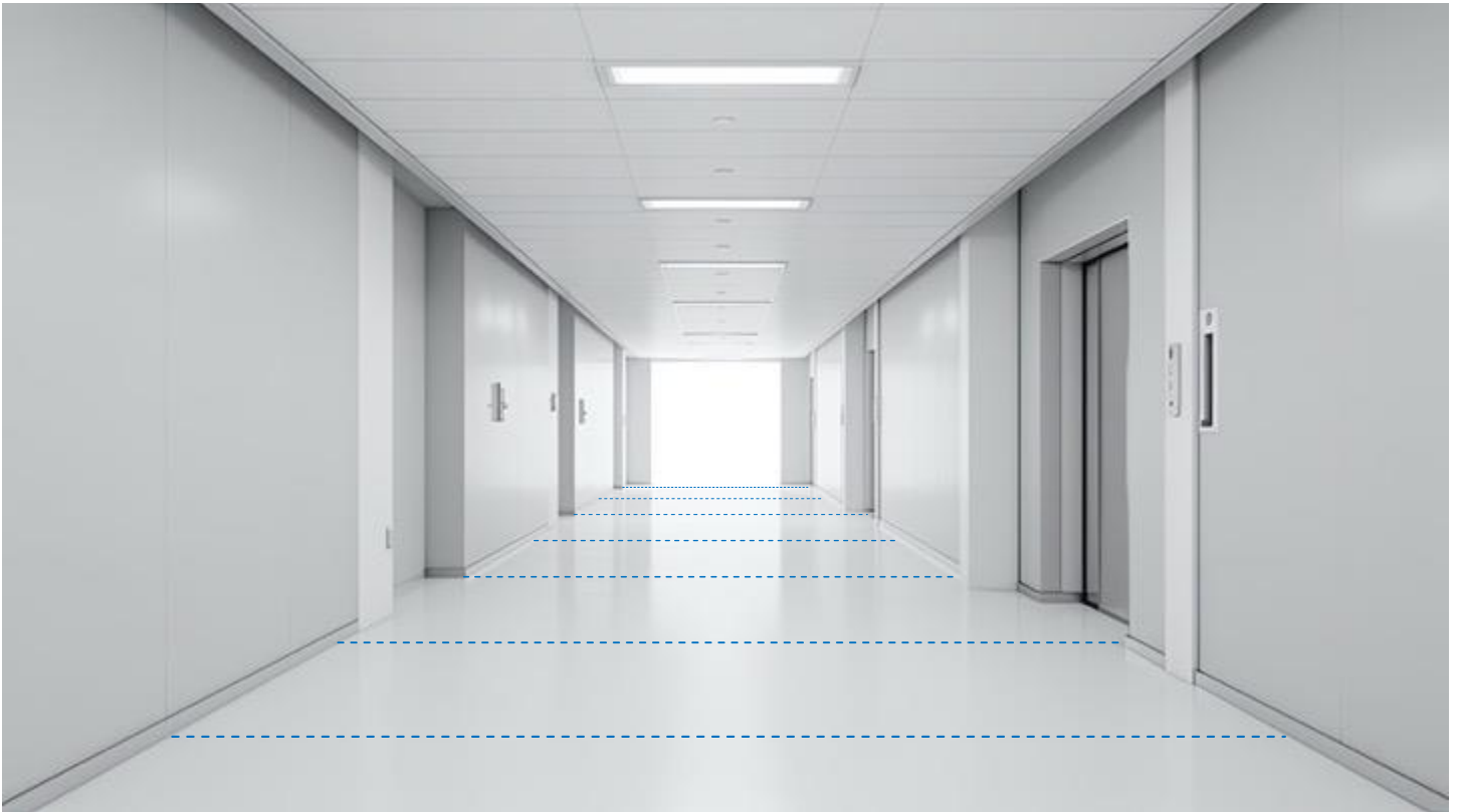
Figure 15 - Always establish proper seam placement and install rolls and cuts in consecutive sequential order.
