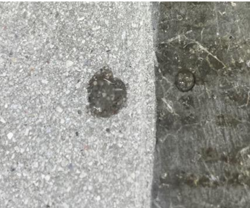
Figure 12 - Check for absorbency using methods outlined in ASTM F3191
