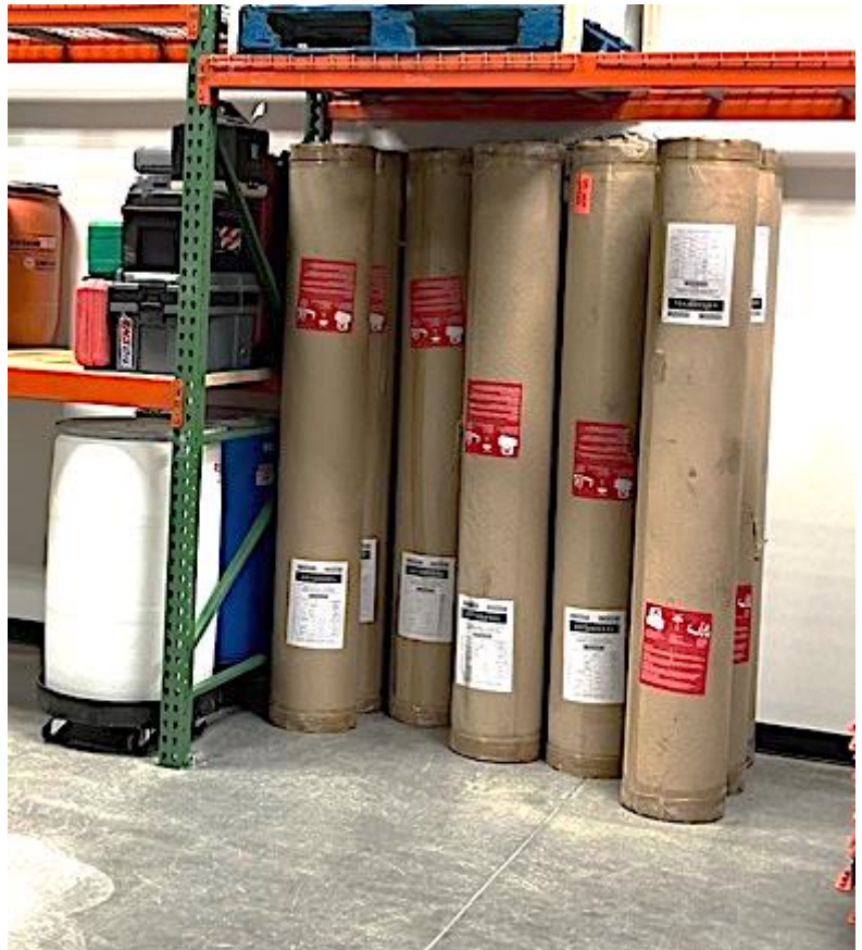
Figure 1 - Rolls should always be stored vertically.
